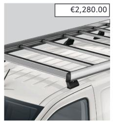
ALUMINIUM ROOF PLATFORM COMPACT (LWB) Heavy duty aluminium platform with integrated roller bar to facilitate loading.
