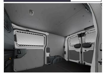
The finishing touch to your panel van is the insulated roof panel. It's designed to match the plastic panels made especially for your Proace van.
